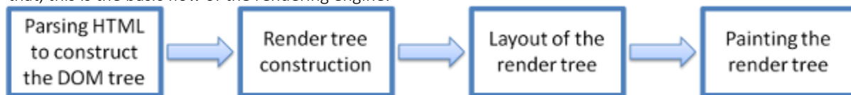
Figure : Rendering engine basic flow
