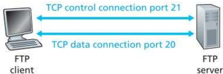
Fig: Control and data connections
